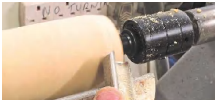
▲ Pic.7 The tool can be used for shaping curves but make sure the bevel remains in contact with the timber, as the tool has the tendency to run back if you go onto the edge
